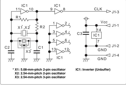
Figure 5.2 Circuit of the oscillator board (OSC-2)
